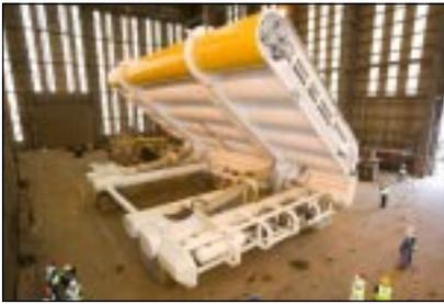
The wave power converter Oyster (full-scale) in open position
