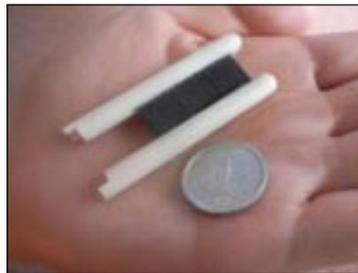
External appearance of a micro SOFC module (fuel stack at the centre)
