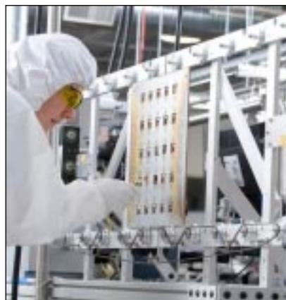
New thin films cells being readied for testing at Sencera
