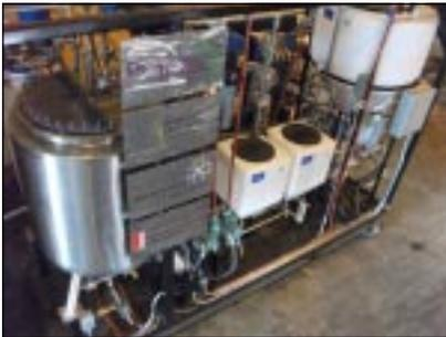
*The enzymatic biodiesel pilot plant developed by Piedmont Biofuels*
