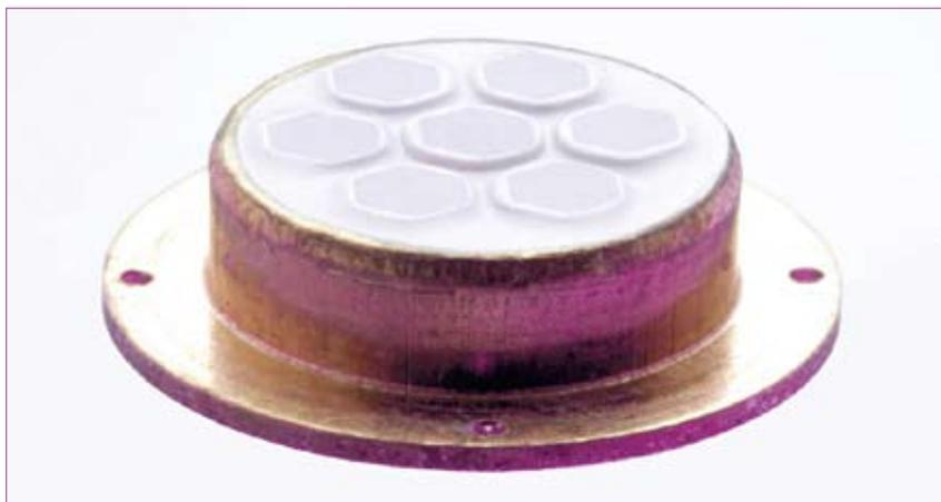
This mechanically stabilized nanoporous filter membrane exhibits a regular pore structure. At the same time, the pore size distribution is very tight and even. (© Fraunhofer IWM)
