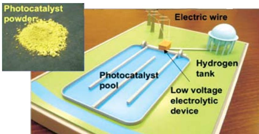
New high-performance photocatalyst (upper left) and an overall model of the photocatalyst-electrolysis hybrid system
