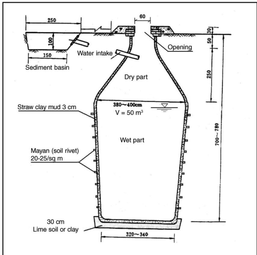
Figure 2: Water cellar with cement mortar pasted wall and concrete dome structure
