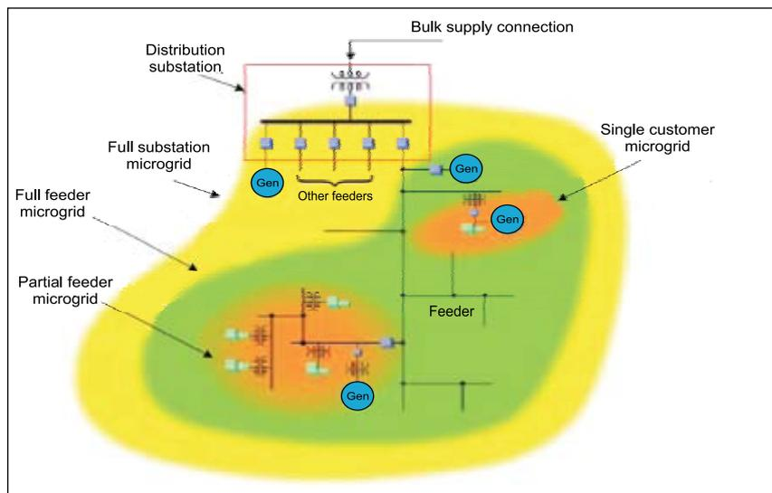
Fig. 1. Micro-grid structure
