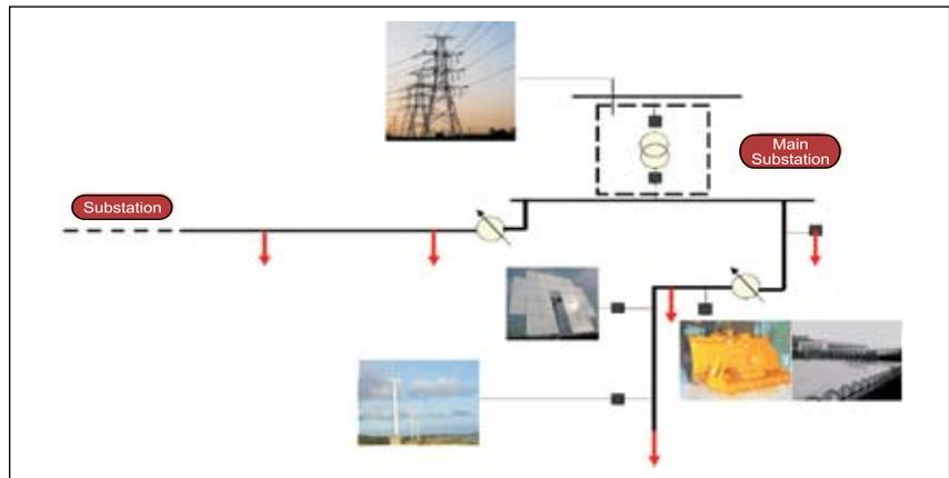
Fig. 2. Schematic diagram of utility micro-grid
