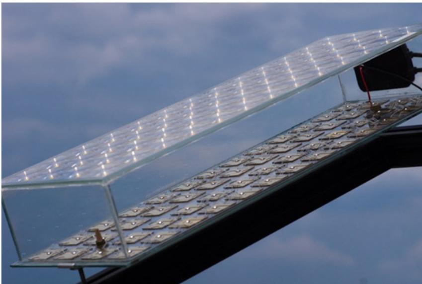
**Newest FLATCON® concentrator module with an efficiency of 36.7%. ©Fraunhofer ISE (Credit: Alexander Wekkeli)**
