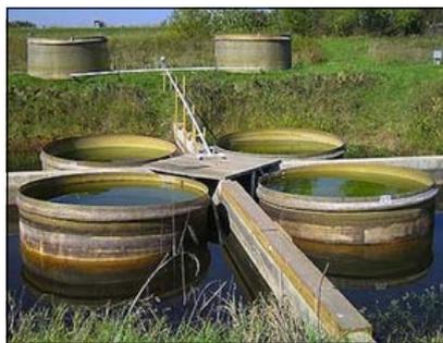
*Demonstration of integrated wastewater algae-to-biocrude process*
